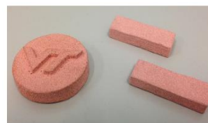
Fig. 8: Sintered copper part samples (AcuPowder 153A copper powder sintered in pure hydrogen at 1000 °C for 8 hours) [47].
